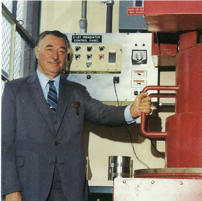
The late Dr. Eugen Wierbicki, with the equipment he used to treat foods with ionizing energy at the U.S. Department of Agriculture's Eastern Regional Research Center in Philadelphia.
