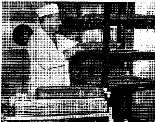
The late Dr. Eugen Wierbicki demonstrating the use of a cook-house to inactivate autolytic enzymes in beef before sterilization with ionizing energy. Photograph courtesy of Edward S. Josephson, Department of Chemical Engineering, Massachusetts Institute of Technology.
