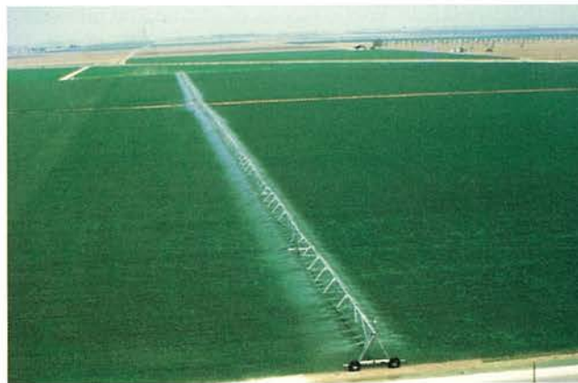
During the Dust Bowl era, wind erosion buried equipment. Modern lateral-move sprinkler irrigating Nebraska crops. Credits: Soil Conservation Service, U.S. Department of Agriculture (top) and Valmont Industries, Inc. (bottom).
