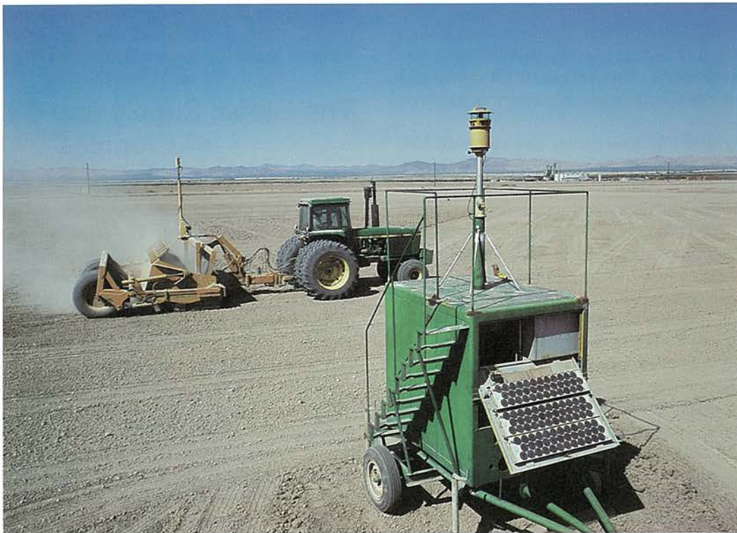
The leveling of land to speed the advance of irrigation water across a field and so increase the water use efficiency. The leveling is guided by a laser seen in the foreground of the lower photo. The laser beams can be seen in the upper photo. Credits: Robert C. Bjork, ARS, U.S. Department of Agriculture (top) and A. R. Dedrick, U.S. Water Conservation Laboratory, Phoenix, Arizona (bottom).
